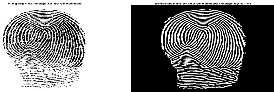
Figure 4: Fingerprint enhancement using STFT analysis. The left shows the original image which is which is Image 1 in [8]. The right shows the binarized enhanced image using STFT.
