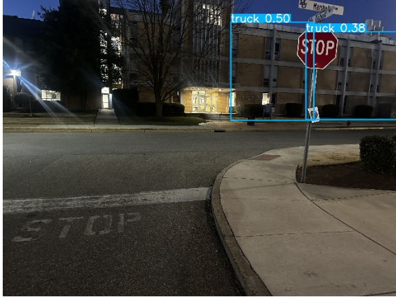
Stop sign with the adversarial patch with 2 distinct confidences of being a truck located where the stop sign is.
